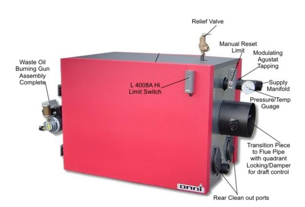
Figure 6 - Boiler (OWB-35 & OWB-50)
